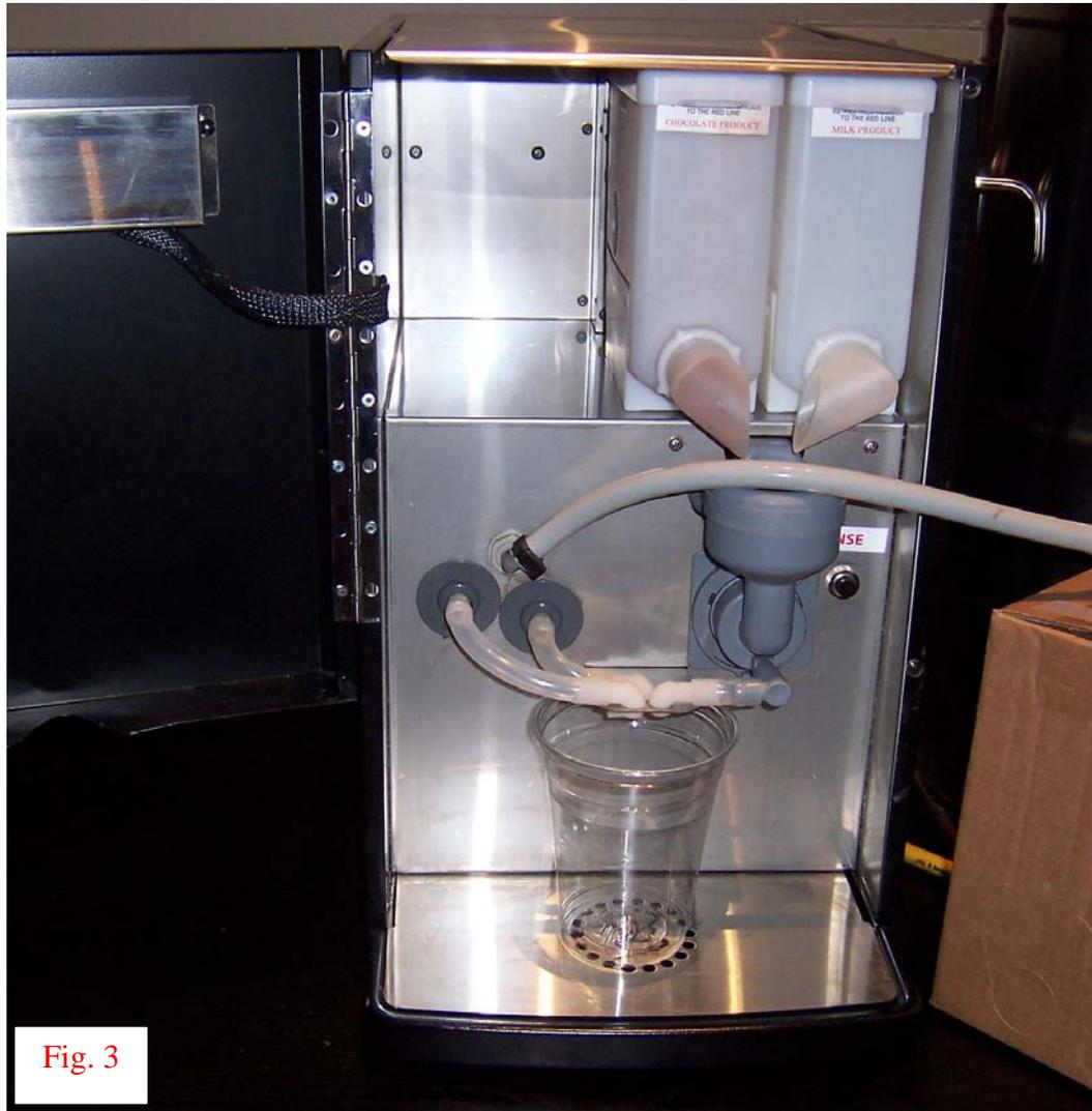
2. Place an empty container in the dispense area of the machine as shown in **figure 3**.
