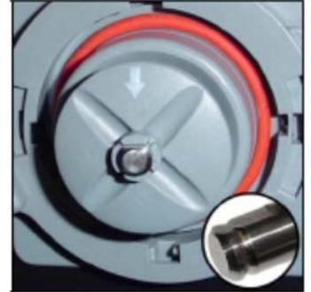
When installing the impeller onto the shaft, make certain that it clicks into position (figure2). If the impeller is not pushed in far enough (figure 1), it will rub on the whipper chamber and eventually seize. If it is installed too far on the shaft (figure 3), it may rub on the whipper base and eventually seize. In both cases, the product will not mix properly and may cause a blockage in the powder system outlet hose.
