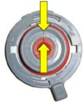
After replacing the seal, inspect the larger rubber O-ring [767390] in the base for cuts, nicks, and deformities. If the O-ring appears damaged in any way, it should be replaced.
