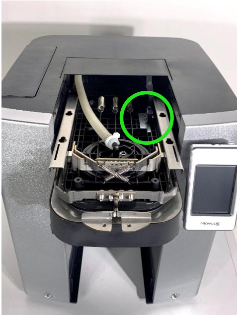
The Limit Switch Bracket is installed onto the Brew Mech Upper.
