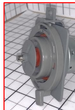
Impeller pushed on too far
