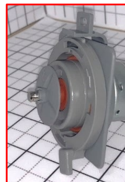
Impeller pushed on too far
