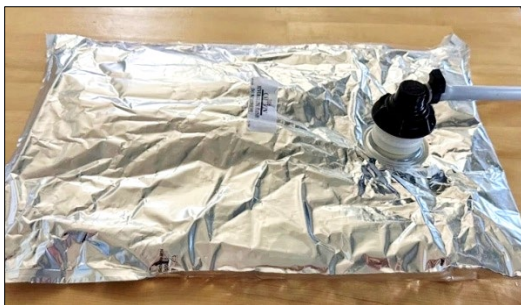
5. Connect tube to BIB cleaning / flushing solution
