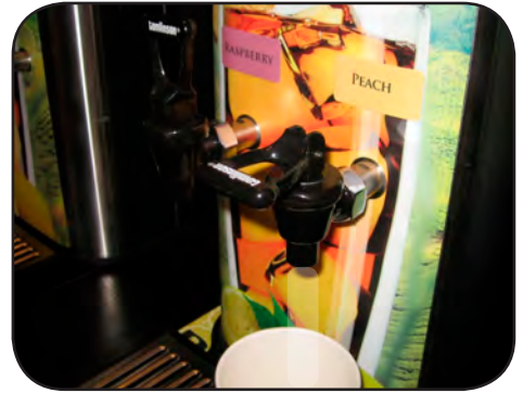
Flush system for 2 minutes or until the discharged solution runs clear.
