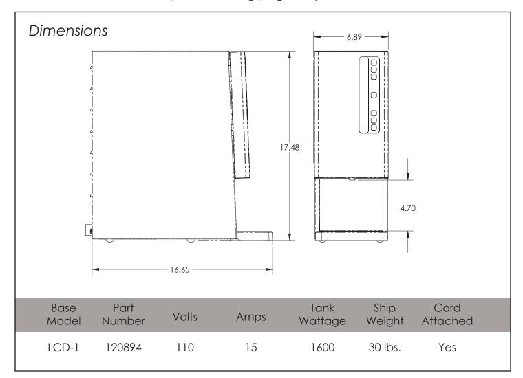
**Electrical:** 120 V models are 2 wires plus ground service rated 120V, single phase, 60Hz.
