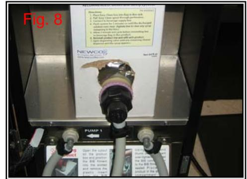
Disconnect sanitizing solution from Pump 1 and connect to the BIB connector for PUMP 2 as shown figures 7 & 8.
