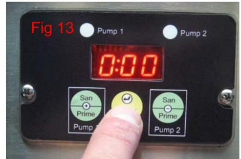
7. Press “Enter” to save and proceed to the next set-up programming option. SEL will appear on the display.
