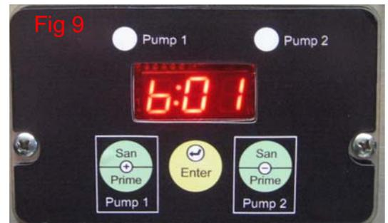
2. Press Enter. The number "1" and the current speed for pump 1 will appear in the display. As shown in figure 10.
