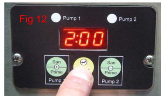
5. Using the + or - button, set Pump 2 speed for the desired ratio using Chart A as a guide. (If blending 2 products, use Chart B as a guide.) Refer to fig. 11 – step 3.
