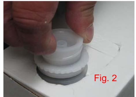
Using finger and thumb only to prevent over-tightening, thread the BIB connector on to the BIB fitment until seated as shown in figure 3.
