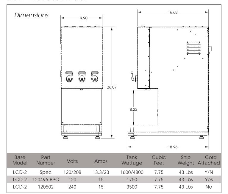
**Electrical:** 120 V models are 2 wires plus ground service rated 120V, single phase, 60Hz. 120/240 V, single phase, 60Hz.
