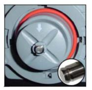
• When installing the impeller onto the shaft, make certain that it clicks into position (figure2). If the impeller is not pushed in far enough (figure 1), it will rub on the whipper chamber and eventually seize. If it is installed too far on the shaft (figure 3), it may rub on the whipper base and eventually seize. In both cases, the product will not mix properly and may cause a blockage in the powder system outlet hose.
