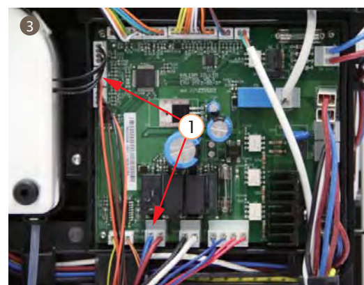
3. Pull out motor group terminal from PCBA and separate with cable rack
