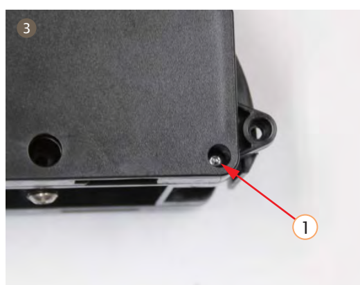
3. Disassemble the 4 screws from the left and right cover
