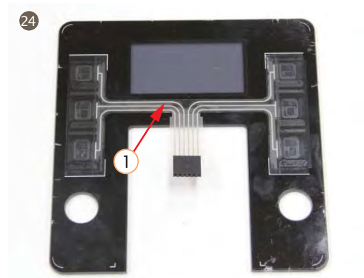
24. Take out ITO which stucked to touch screen
