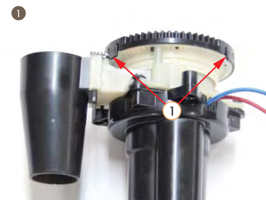
1. Disassemble the 3 hooks from the grinder adjustment sector and take out the grinder adjustment sector
