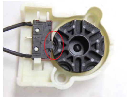
6. Separate dispenser valve from sheave permanent seat, take out sheave and disassemble microswitch.
