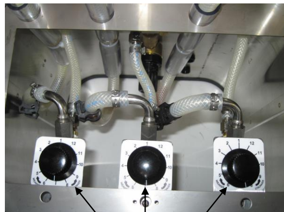
After Access Panel Is Removed Adjustment Dials Are Accessible From The Top Side.
