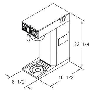
STYLE: Automatic BREW OPERATIONS: Analog / Digital timer HEATING SYSTEM: Tank Reservoir WATER DELIVERY: Displacement TANK SYSTEM: Open VOLTAGE: 120V or 120V/240V Only CABINET: Semi-Modular ENERGY SMART: Yes FLOW REGULATION: PDS BACKUP POUR IN: No FAUCET: Gravity
