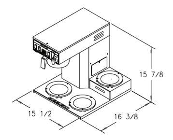
STYLE: Automatic BREW OPERATIONS: Analog / Digital timer HEATING SYSTEM: Tank Reservoir WATER DELIVERY: Displacement TANK SYSTEM: Open VOLTAGE: 120V or 120V/240V Only CABINET: Semi-Modular ENERGY SMART: Yes FLOW REGULATION: PDS BACKUP POUR IN: No FAUCET: Gravity
