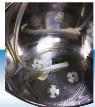
Ozone injector in cold water reservoir
