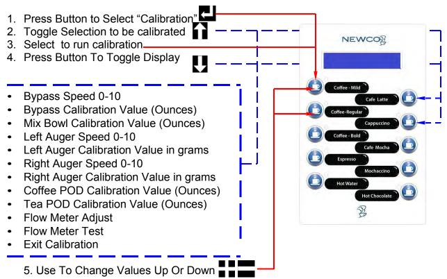
NOTE: SHOULD THE COFFEE OR TEA VOLUME NEED ADJUSTMENT, A SMALL VOLUME CAN BE ADDED OR SUBRACTED BY ADJUSTING THE "FLOWMETER ADJ" VALUE + OR -
