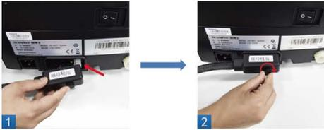
Step 3: Put the other end onto the connection place of fridge lift side. Insert the white connector of the line first, then put on the whole end, and tighten the screws.
