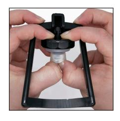
**4.)** Install the no touch handle by placing it on the bonnet in front of the stem. Push up on the seat cup with your thumbs while pushing down on the handle and bonnet with fingers.
