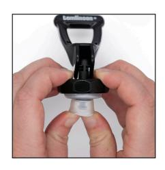
**2.)** Remove existing handle by pushing up on seat cup with thumbs while pushing down on the bonnet and handle with fingers.
