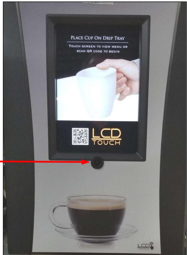
Hold the QR Code up to the scanner on the door. Recipe will begin to brew automatically and shut off once the scanner recognizes the Code.
