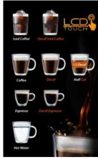
**TAP 3 TIMES ON CENTER OF "D" TO ENTER PROGRAMMING MODE IF A BREWING ICON IS ACCIDENTLY TOUCHED USE THE RETURN ARROW TO TRY AGAIN**
