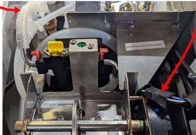
*Note: Shipping Support Bracket must be removed*
