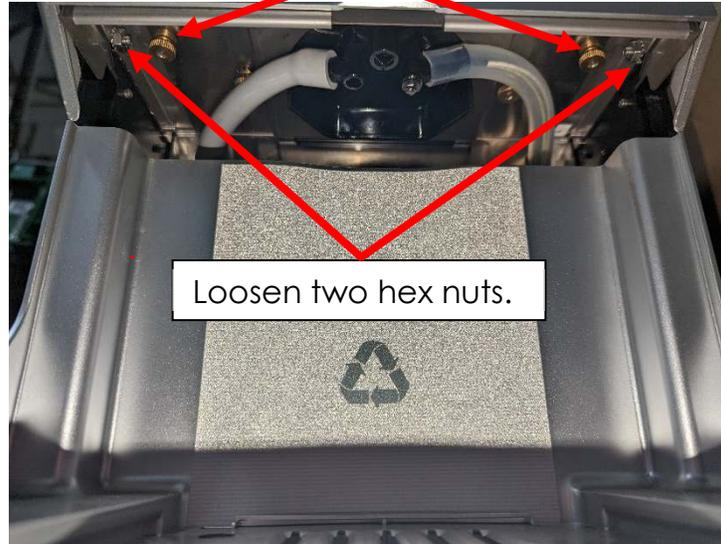
Next, disconnect the water connection, and the harness connection.
