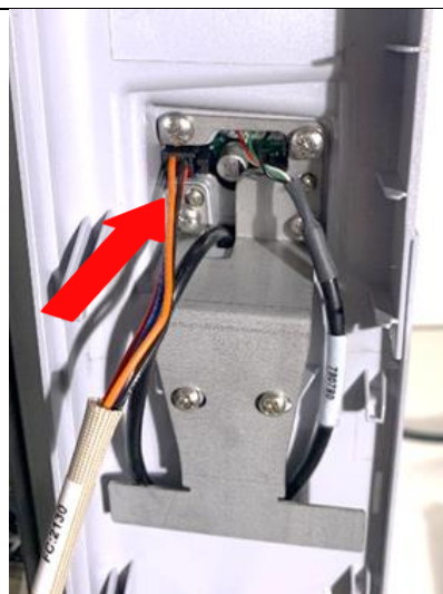
Push wire connection into display board, ensure the locking tab is on the right and the connector is secure.
