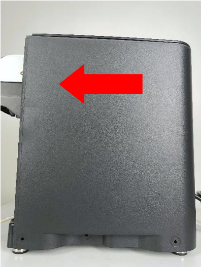
Align upper and lower side panel hooks. Slide right side panel forward about 1/4" to the front of the machine to lock in place.
